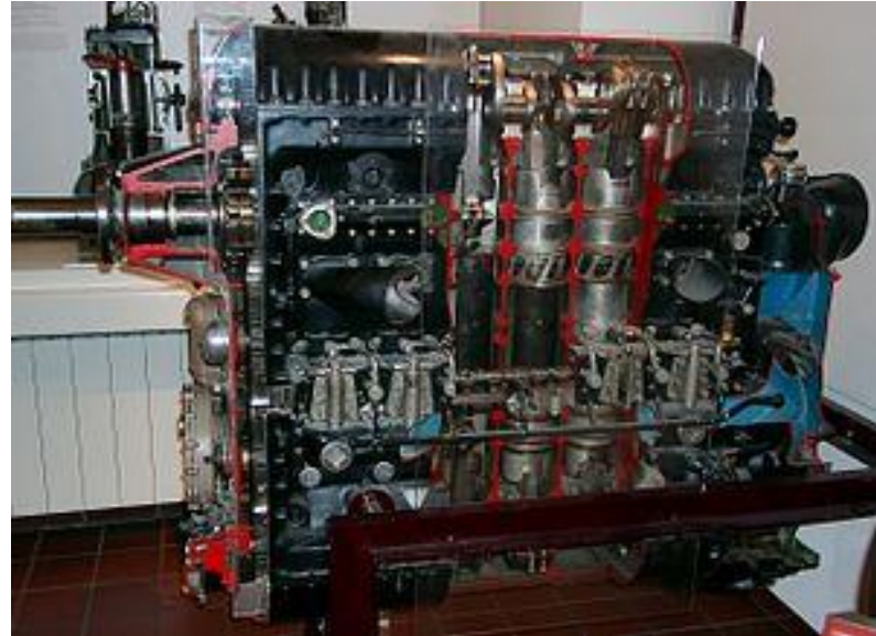
1932 Junkers Jumo 205 diesel aircraft engine
